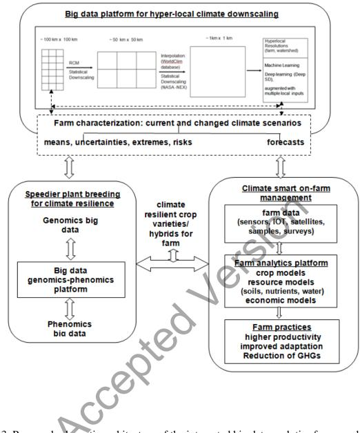
Fig 3: Proposed schematic architecture of the integrated big data analytics framework for climate smart agriculture
